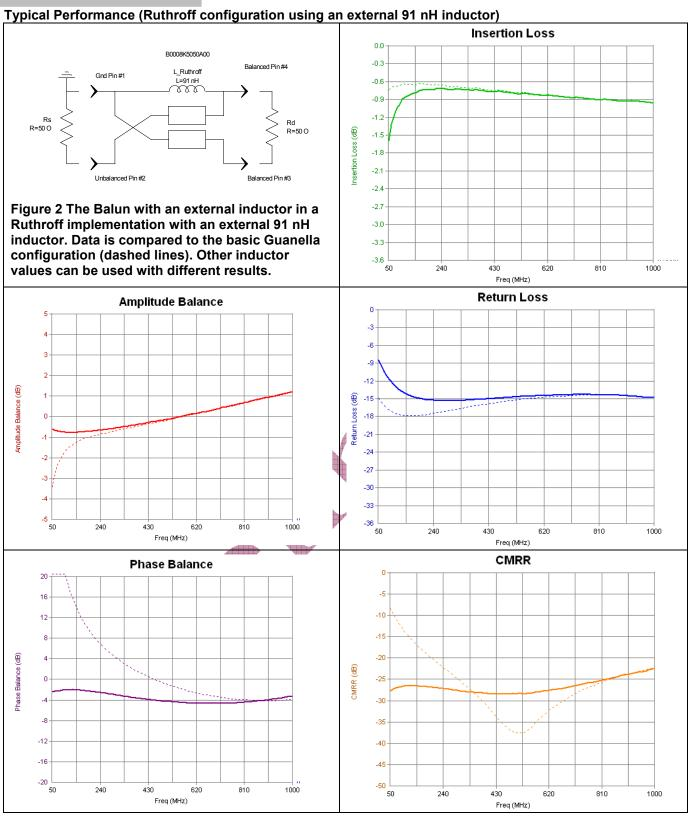
Typical Performance (using DC Block to enhance low frequency insertion & return loss)
