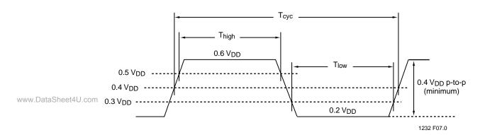
FIGURE 8: LCLK WAVEFORM (LPC MODE)
