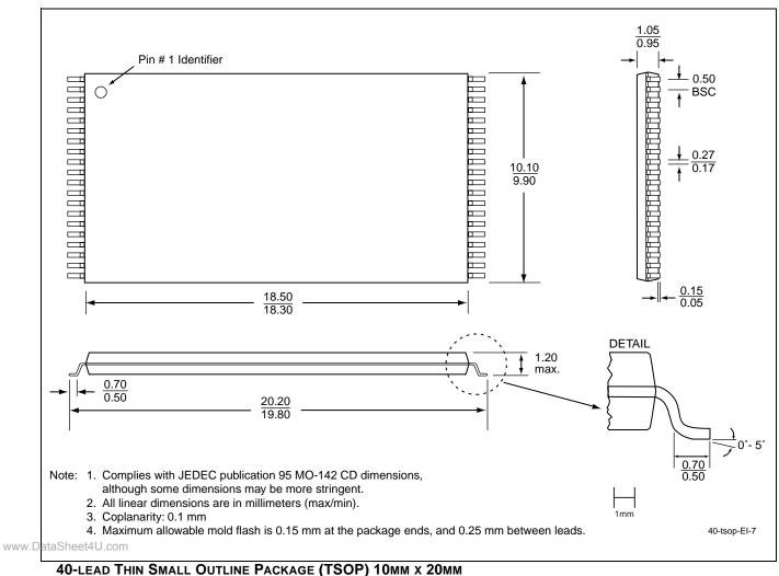
40-LEAD THIN SMALL OUTLINE PACKAGE (TSOP) 10MM x 2 SST PACKAGE CODE: EI
