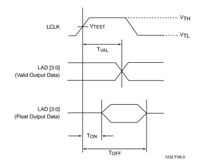
FIGURE 9: OUTPUT TIMING PARAMETERS (LPC MODE)
