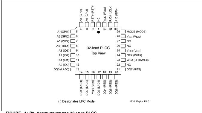
FIGURE 1: PIN ASSIGNMENTS FOR 32-LEAD PLCC
