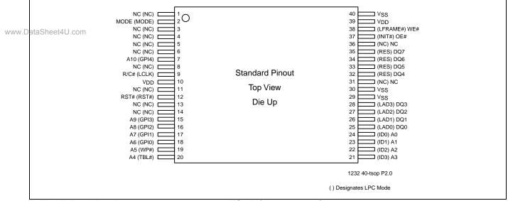
FIGURE 2: PIN ASSIGNMENTS FOR 40-LEAD TSOP (10MM X 20MM)
