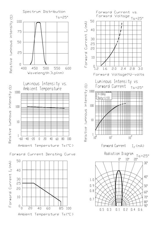
Everlight Electronics Co., Ltd. Device No. : SZDLE-952-030 http://www.everlight.com Prepared date: 19-Apr-2005 Rev. 1Page: 5 of 10Prepared by: bianchangyou
