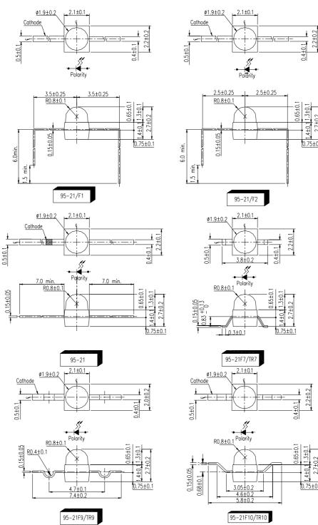
**Note:** The tolerances unless mentioned is  $\pm 0.1$ mm ,Unit = mm
