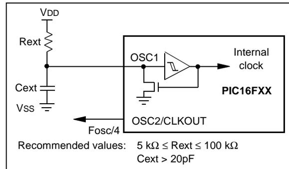
**Note:** When the device oscillator is in RC mode, do not drive the OSC1 pin with an external clock or you may damage the device.
