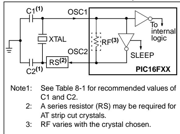
The PIC16F8X oscillator design requires the use of a parallel cut crystal. Use of a series cut crystal may give a frequency out of the crystal manufacturers specifications. When in XT, LP or HS modes, the device can have an external clock source to drive the OSC1/CLKIN pin (Figure 8-4).
