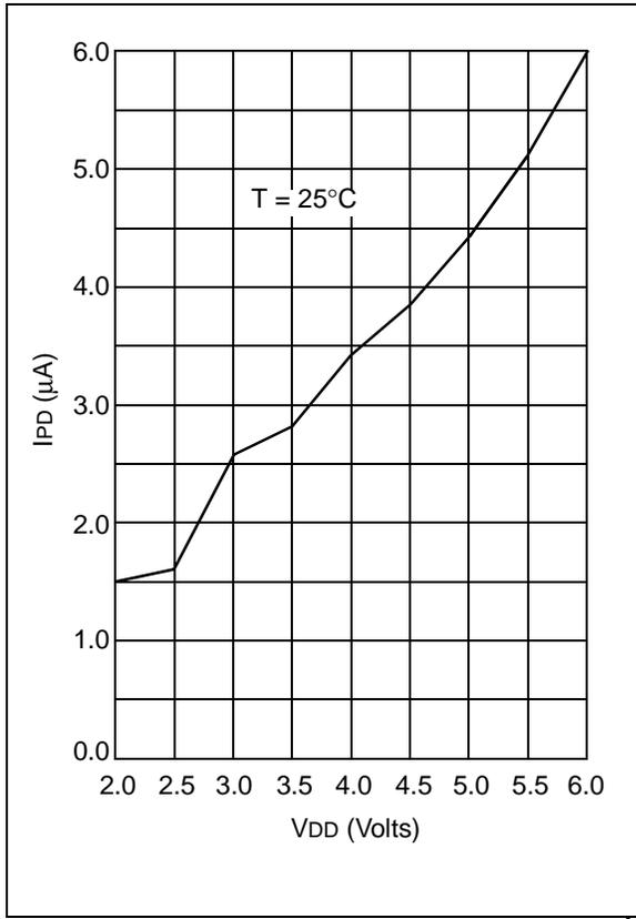
**FIGURE 13-6: TYPICAL  $I_{PD}$  vs.  $V_{DD}$ , WATCHDOG ENABLED**
