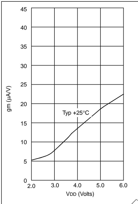
FIGURE 13-16: TRANSCONDUCTANCE (gm) OF XT OSCILLATOR vs. VDD
