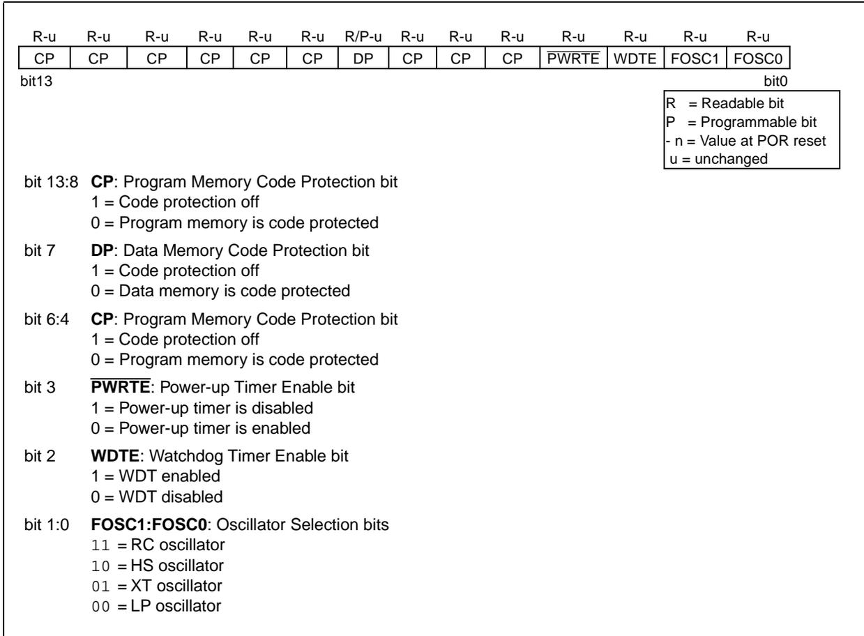
**FIGURE 8-2: CONFIGURATION WORD - PIC16F83 AND PIC16F84**
