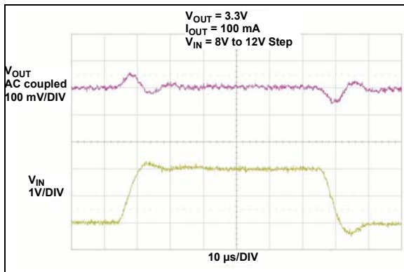
FIGURE 2-20: Line Transient Response.
