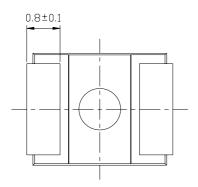
For reflow soldering (propose)
