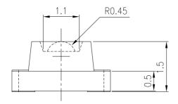
For reflow soldering (propose)
