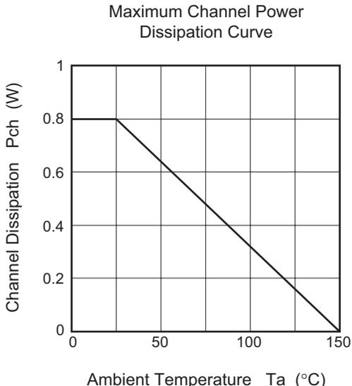
\*When using the glass epoxy board (FR-4: 40 × 40 × 1 mm)
