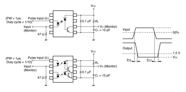
Remark CL is approximately 15 pF which includes probe and stray wiring capacitance.
