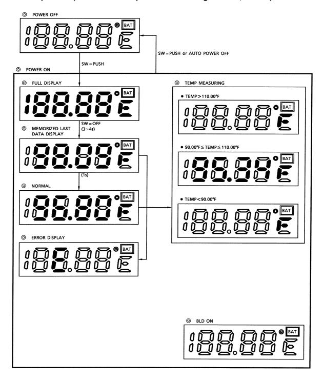
3. Switch Operation (stable detection informing function, unit: °C)
