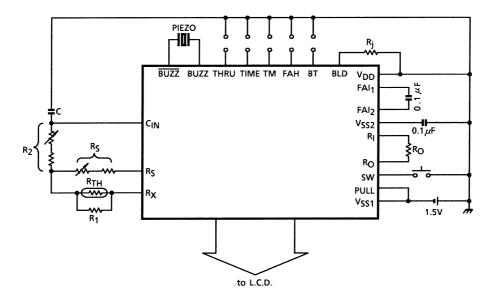
It is desirable to use C,  $R_1$ ,  $R_2$  and  $R_S$  having the satisfactory temperature characteristic. It is desirable to minimize the range of variable resistance of  $R_2$  and  $R_S$  could as possible.
