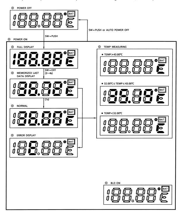
2. Switch Operation (in case of the elapsed time informing function, unit: °F)
