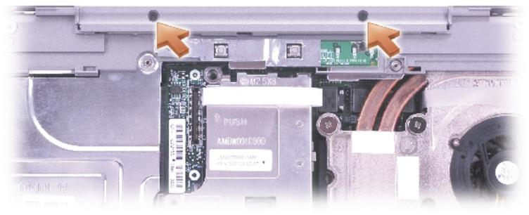
10. Disconnect the touch pad connector from the system board.
