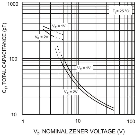
Fig. 5 Total Capacitance vs Nominal Zener Voltage
