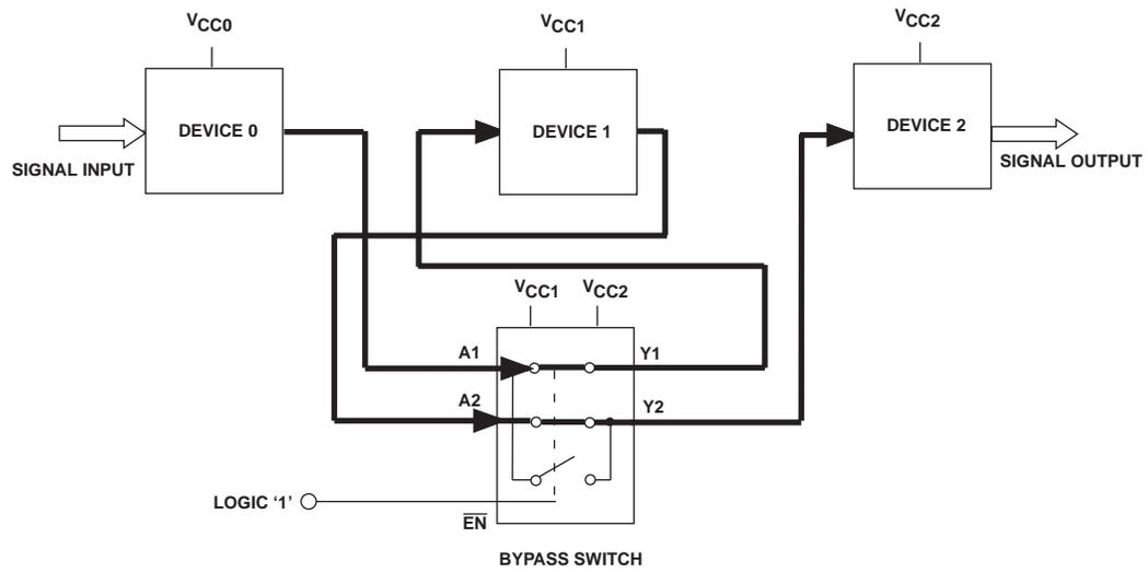
Figure 4. Bypass Switch in Normal Mode
