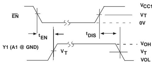
Figure 2. Y1 Enable and Disable Times
