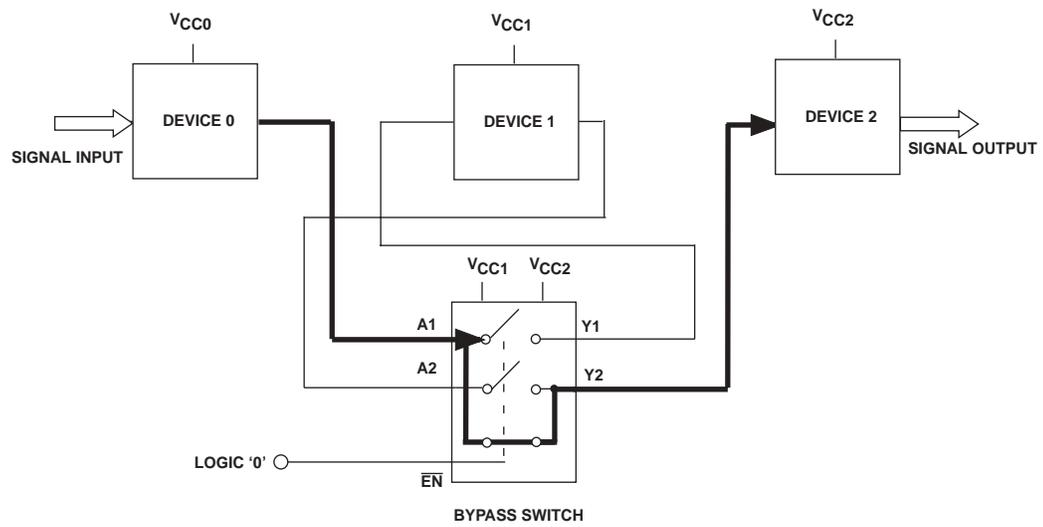
Figure 5. Bypass Switch in Bypass Mode
