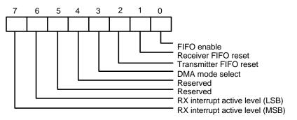
Notes: Bit 6, 7: These two bits are used to set the active level for the receiver FIFO interrupt. For example, if the interrupt active level is set as 4 bytes, once there are more than 4 data characters in the receiver FIFO, the interrupt will be activated to notify the CPU to read the data from the FIFO.
