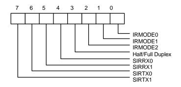
Notes: SIRTX1 SIRTX0 (Bit 7, 6): These two bits select IRTX pin in the IR function. 00 or 11 IRTX2 (Pin 2, PDBDIR) 01 IRTX1 (Pin 43, SOUTB) 10 IRTX3 (Pin 95, nCS1) During the power-on reset, the default value is 00.
