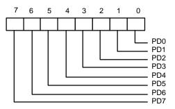
When accesses are made to any EPP data port, the contents of DB0-DB7 are buffered (non-inverting) and output to the ports PD0-PD7 during a write operation. The leading edge of  $\overline{IOW}$  causes
