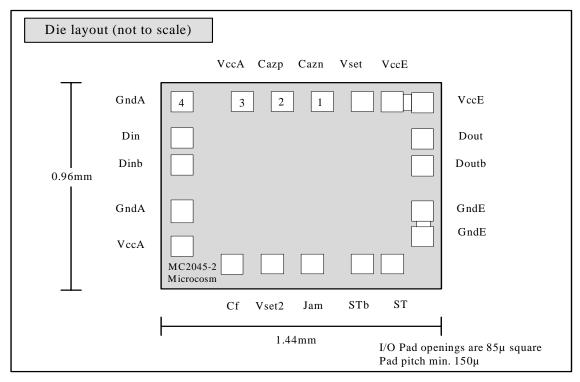
$V_{\text{SET}}$  and  $V_{\text{SET2}}$  are alternative inputs to the same 'Vset' function. Connect one or other, not both.
