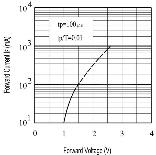
**Typical Electro-Optical Characteristics Curves**
