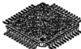
48-PIN PLASTIC FLAT PACK (FPT-48P-M02)
