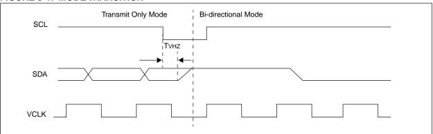
FIGURE 3-2: DATA TRANSFER SEQUENCE ON THE SERIAL BUS
