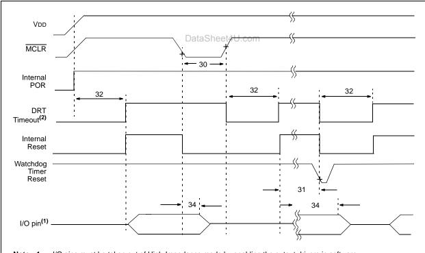
Note 1: I/O pins must be taken out of High-Impedance mode by enabling the output drivers in software.
