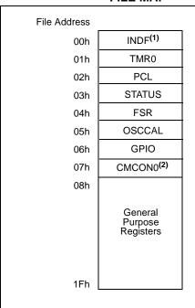
Note 1: Not a physical register. See Section 4.9 "Indirect Data Addressing: INDF and FSR Registers".
