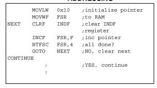
The FSR is a 5-bit wide register. It is used in conjunction with the INDF register to indirectly address the data memory area.
