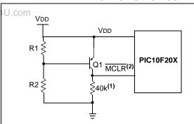
Note 1: This brown-out circuit is less expensive, although less accurate. Transistor Q1 turns off when VDD is below a certain level such that:
