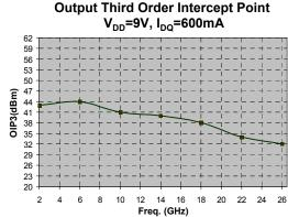
\* Measured data includes effect of two parallel RF input/output bond wires
