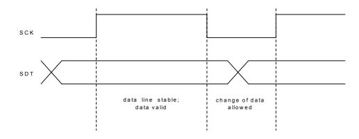
Figure 24. Bit transfer timing
