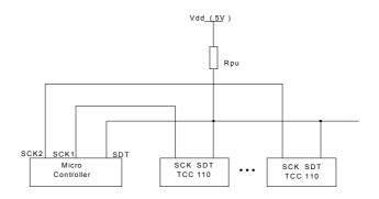
Figure 22: Serial bus configuration
