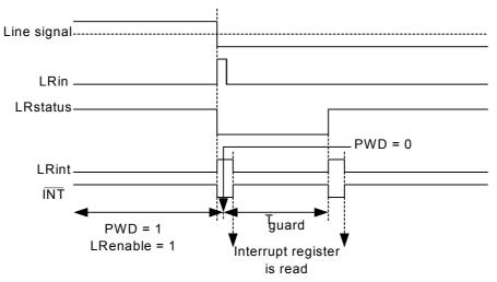
Figure 12 : Behavior of signals on a line reversal
