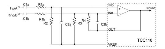
Figure 3. Differential input buffer of the TCC110
