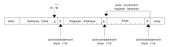
Figure 27: Write sequence of the serial interface
