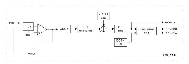
Figure 18: DC measurement block configuration for DC line voltage measurement mode
