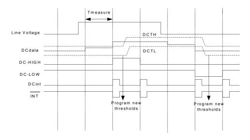
Figure 16: Interrupt generation of the DC voltage measurement block when DC-INT mode = 0
