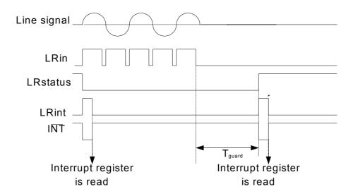
Figure 13: Behavior of signals during ring
