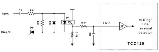
Figure 11. External component to generate LRin
