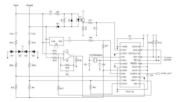
Figure 2. Recommended external components for typical application
