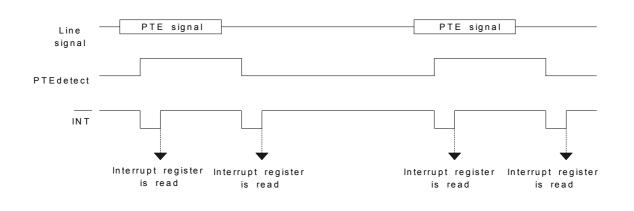
Figure 10: PTE detector operation
