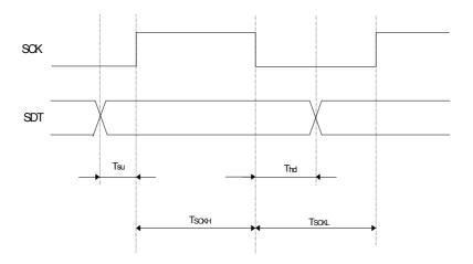
Figure 33: Timing of SCK and SDT during byte transmission
