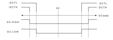
Figure 15: Behavior of DC-HIGH and DC-LOW related to DCdata, DCTH and DCTL
