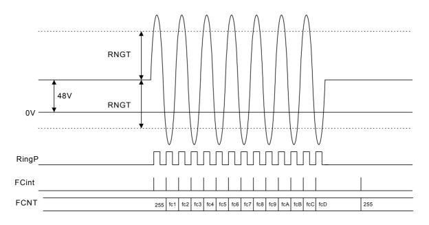
Figure 21: Behavior of RING when a ring occurs on the line (FCint only behaves as shown when FCenable = 1)
