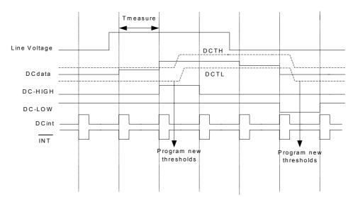
Figure 17: Interrupt generation of the DC voltage measurement block when DC-INT mode = 1
