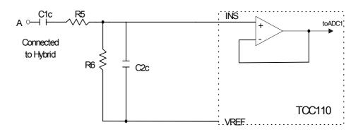
Figure 4. Single ended buffer of the TCC110
