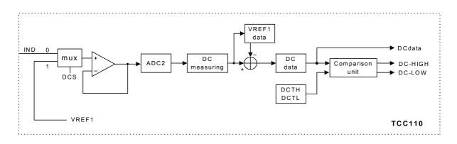
Figure 19: DC Level Detector configuration for reference voltage measurement mode
