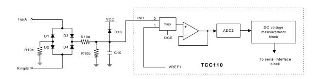
Figure 14: DC voltage measurement block
