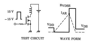
$$\begin{aligned} R_G &= 25~\Omega \\ V_{DD} &= 25~V,~L = 339~\mu H \end{aligned} \qquad E_{AS} &= \frac{1}{2} \cdot L \cdot I^2 \cdot \left( \frac{Bv_{DSS}}{Bv_{DSS} - V_{DD}} \right) \end{aligned}$$
