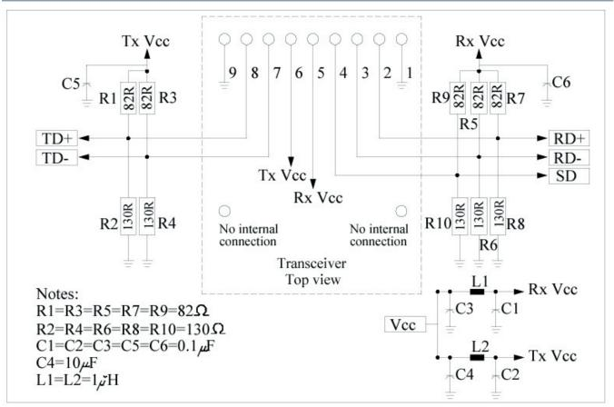
The split-loaded terminations for ECL signals need to be located at the input of devices receiving those ECL signals. The power supply filtering is required for good EMI performance. Use short tracks from the inductor L1/L2 to the module Rx Vcc. A GND plane under the module is required for good EMI and sensitivity performance.
