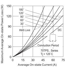
Fig. 4 - On-State Power Loss Characteristics
