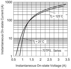
Fig. 7 - On-State Voltage Drop Characteristics
