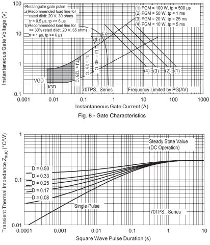
Fig. 9 - Thermal Impedance ZthJC Characteristics
