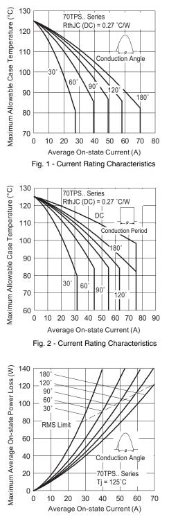
Fig. 3 - On-State Power Loss Characteristics
