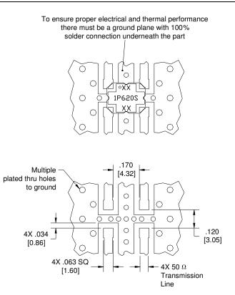
Dimensions are in Inches [Millimeters] 1P620S Rev A Mounting Footprint
