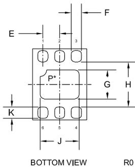
\*Exposed pad P internally connected to pins 2, 3, 4, and 5.
