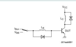
$$V_{CC}=300~V;\,V_{BB}=\,-\,5~V;L_C=200~\mu H;L_B=1\,\mu H$$
