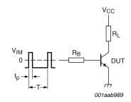
$V_{IM} = -6 \text{ to } +8 \text{ V}; V_{CC} = 250 \text{ V}; t_p = 20 \text{ } \mu\text{s}; \delta = \frac{t_p}{T} = 0.01$  $R_{B}$  and  $R_{L}$  calculated from  $I_{Con}$  and  $I_{Bon}$  requirements.
