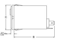
Mounting holes:  $\frac{.13}{3.3}$  Dia. (2) with .23 Dia. x 90° Counter sunk
