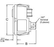
Mounting holes:  $\frac{.13}{3.3}$  Dia. (2) with .23 Dia. x 90° Counter sunk
