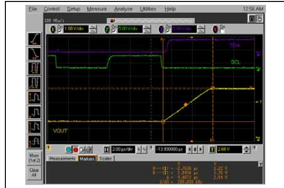
FIGURE 2-98: Half-Scale Settling Time (400h to C00h) (MCP4726).
