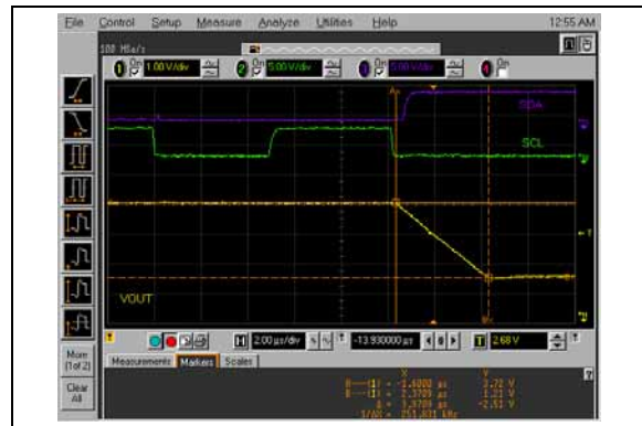
FIGURE 2-99: Half-Scale Settling Time (C00h to 400h) (MCP4726).
