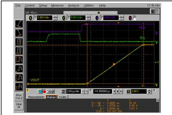
FIGURE 2-96: Full-Scale Settling Time (000h to FFFh) (MCP4726).
