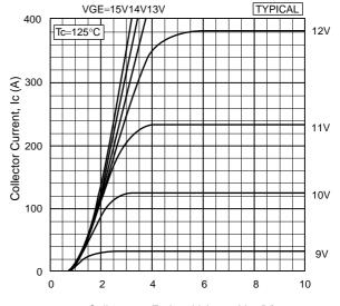
Collector to Emitter Voltage,  $V_{\text{CE}}\left(V\right)$  Collector current vs. Collector to Emitter voltage
