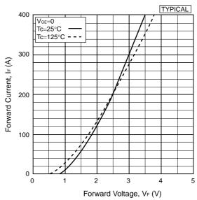
Forward voltage of free-wheeling diode
