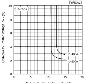
$\label{eq:Gate to Emitter Voltage, VGE (V)} \textbf{Collector to Emitter voltage vs. Gate to Emitter voltage}$
