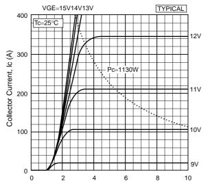
Collector to Emitter Voltage,  $V_{\text{CE}}$  (V) Collector current vs. Collector to Emitter voltage
