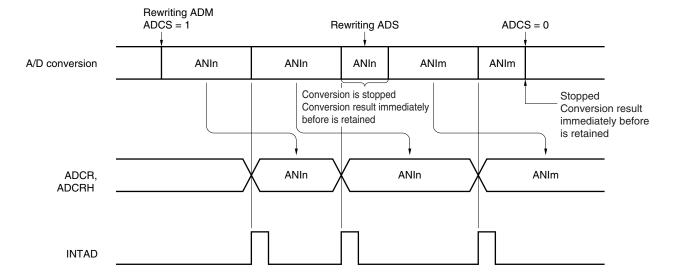
Figure 13-13. A/D Conversion Operation
