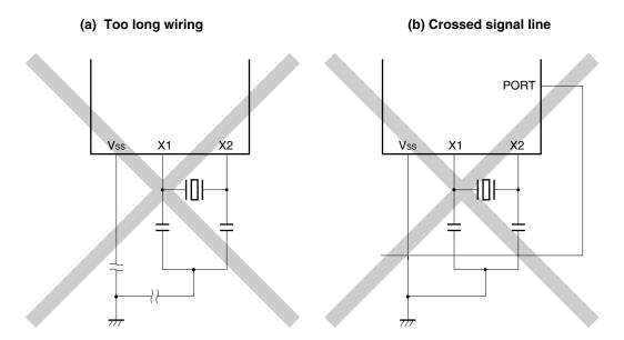
**Remark** When using the subsystem clock, replace X1 and X2 with XT1 and XT2, respectively. Also, insert resistors in series on the XT2 side.
