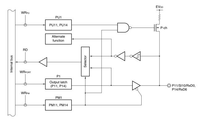
PU1: Pull-up resistor option register 1
