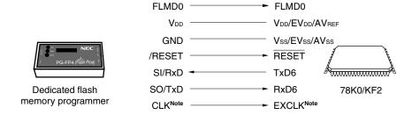
**Note** The above figure illustrates an example of wiring when using the clock output from the PG-FP4 or FL-PR4. When using the clock output from the PG-FPL3 or FP-LITE3, connect CLK to X1/P121 (pin 15), and connect its inverted signal to X2/EXCLK/P122 (pin 14).
