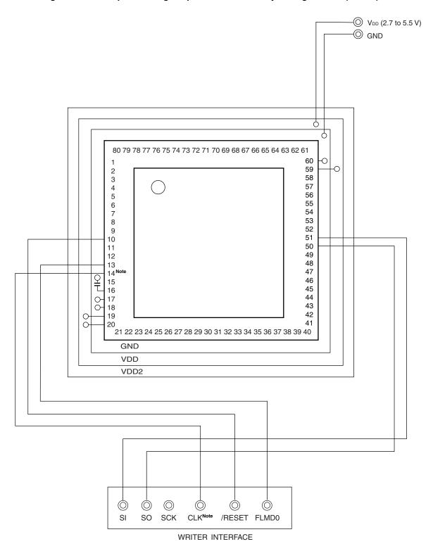
**Note** The above figure illustrates an example of wiring when using the clock output from the PG-FP4 or FL-PR4. When using the clock output from the PG-FPL3 or FP-LITE3, connect CLK to X1/P121 (pin 15), and connect its inverted signal to X2/EXCLK/P122 (pin 14).
