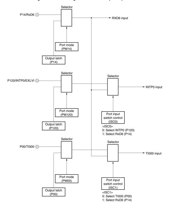
Figure 15-3. Port Configuration for LIN Reception Operation
