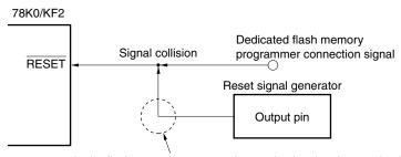
In the flash memory programming mode, the signal output by the reset signal generator collides with the signal output by the dedicated flash memory programmer. Therefore, isolate the signal of the reset signal
