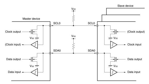
Figure 18-11. Pin Configuration Diagram
