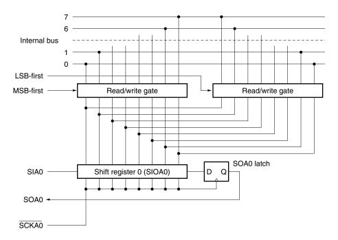
Figure 17-12. Transfer Bit Order Switching Circuit
