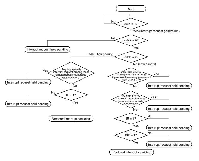
Figure 20-7. Interrupt Request Acknowledgment Processing Algorithm
