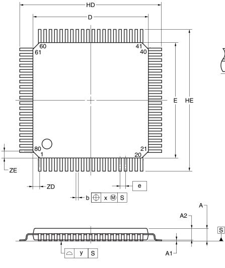
**NOTE**Each lead centerline is located within 0.13 mm of its true position at maximum material condition.
