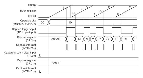
This is a timing example where an edge is not input to the Tl00n pin, in an application where the count value is captured to CR00n when the rising or falling edge of the Tl01n pin is detected.
