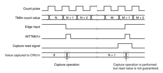
Figure 7-61. Timing of Holding Data by Capture Register
