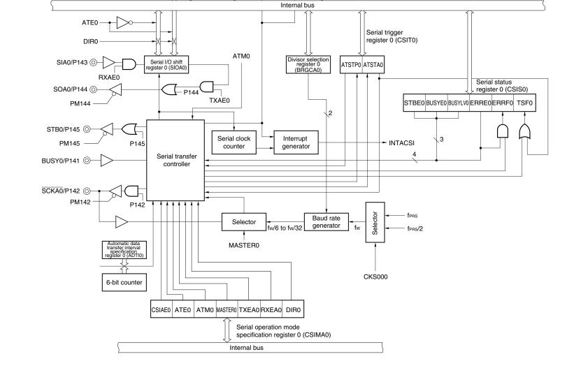
Figure 17-1. Block Diagram of Serial Interface CSIA0
