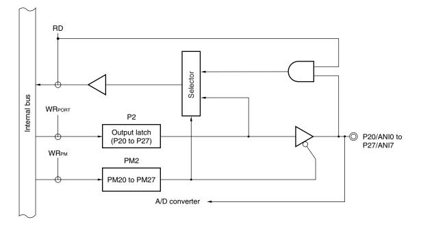
Figure 5-11. Block Diagram of P20 to P27
