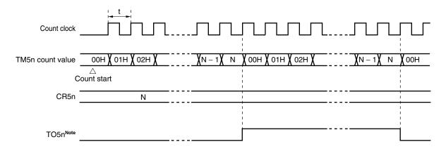
**Note** The initial value of TO5n output can be set by bits 2 and 3 (LVR5n, LVS5n) of 8-bit timer mode control register 5n (TMC5n).
