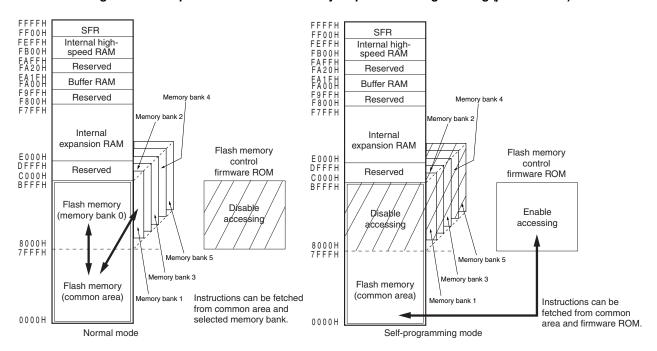
Figure 27-15. Operation Mode and Memory Map for Self-Programming (μPD78F0547)
