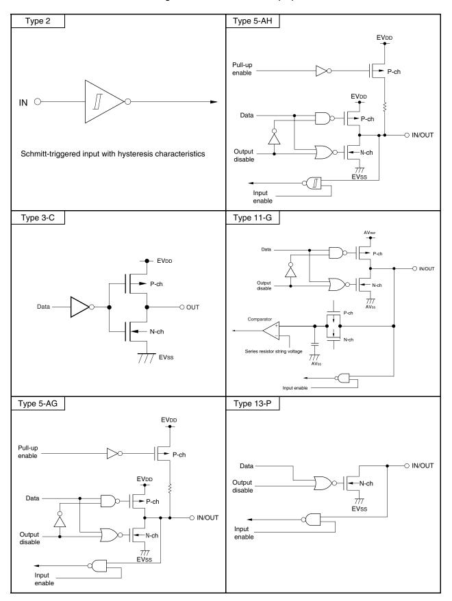
Figure 2-1. Pin I/O Circuit List (2/2)
