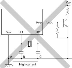
(d) Current flowing through ground line of oscillator
