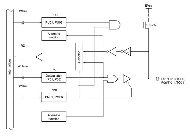
PU0: Pull-up resistor option register 0
