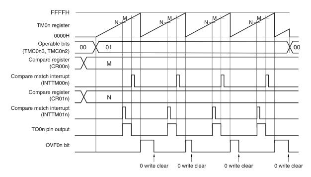
This is an application example where two compare registers are used in the free-running timer mode.
