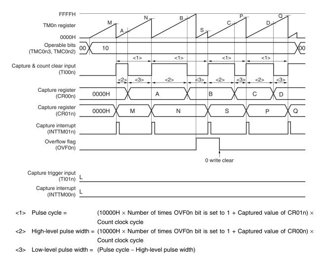
Figure 7-56. Example of Register Settings for Pulse Width Measurement (1/2)
