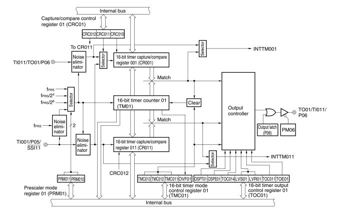
Figure 7-2. Block Diagram of 16-Bit Timer/Event Counter 01
