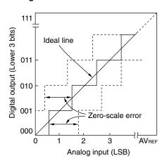
Figure 13-18. Integral Linearity Error
