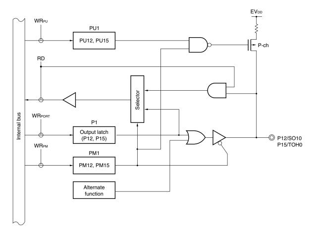
PU1: Pull-up resistor option register 1
