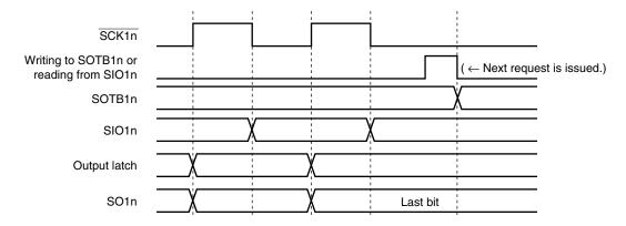
Figure 16-12. Output Value of SO1n Pin (Last Bit) (2/2)
