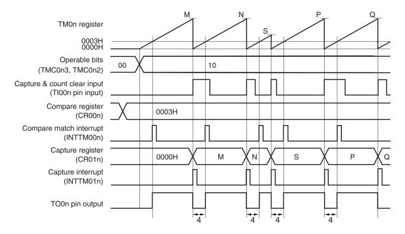
This is an application example where the width set to CR00n (4 clocks in this example) is to be output from the TO0n pin when the count value has been captured & cleared.
