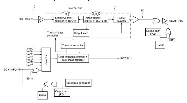
Figure 16-2. Block Diagram of Serial Interface CSI11
