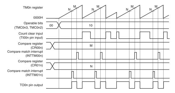
(a) and (b) differ as follows depending on the setting of bit 1 (TMC0n1) of the 16-bit timer mode control register 0n (TMC0n).
