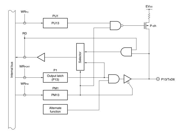
PU1: Pull-up resistor option register 1
