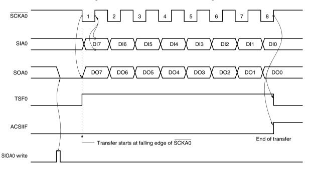
Figure 17-10. 3-Wire Serial I/O Mode Timing
