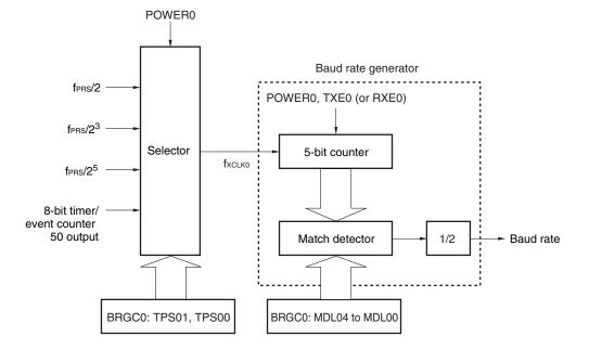
Figure 14-11. Configuration of Baud Rate Generator
