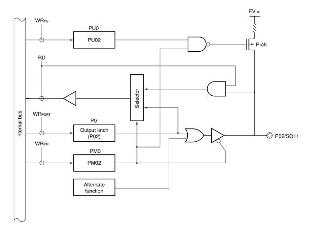
PU0: Pull-up resistor option register 0
