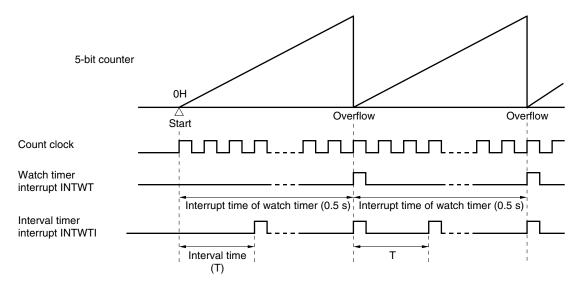
Figure 10-3. Operation Timing of Watch Timer/Interval Timer
