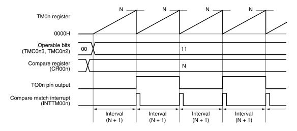
Figure 7-22. Example of Register Settings for Square-Wave Output Operation
