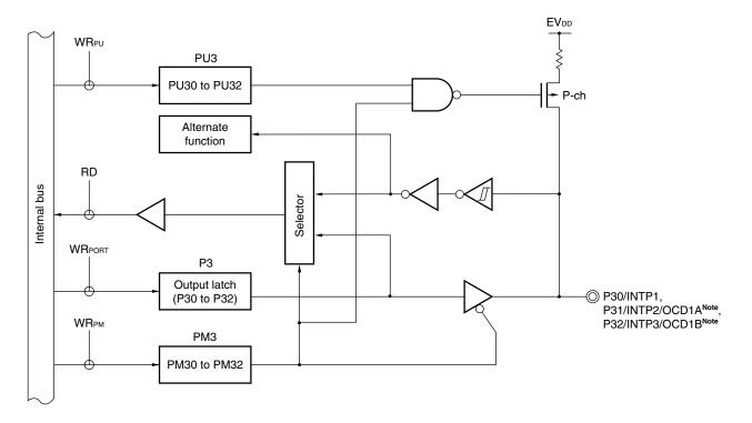
PU3: Pull-up resistor option register 3
