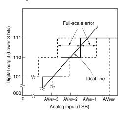
Figure 13-19. Differential Linearity Error
