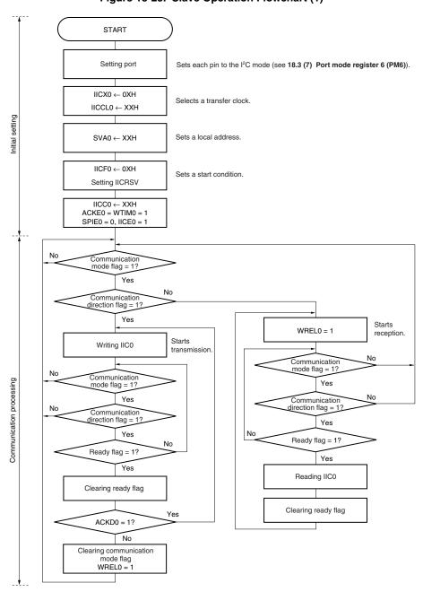
Figure 18-25. Slave Operation Flowchart (1)
