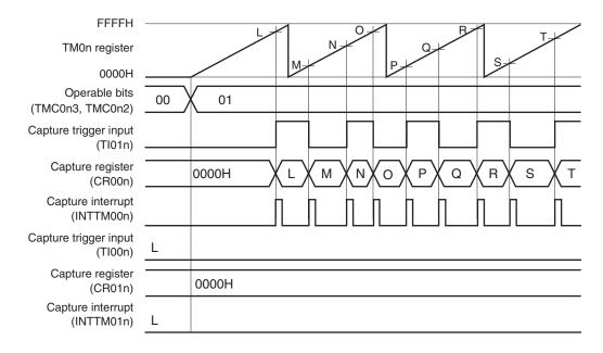
This is an application example where both the edges of the Tl01n pin are detected and the count value is captured to CR00n in the free-running timer mode.
