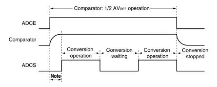
**Note** To stabilize the internal circuit, the time from the rising of the ADCE bit to the falling of the ADCS bit must be 1  $\mu$ s or longer.
