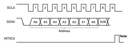
**Note** INTIIC0 is not issued if data other than a local address or extension code is received during slave device operation.
