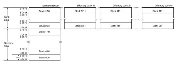
Correspondence between the address values and block numbers in the flash memory are shown below.
