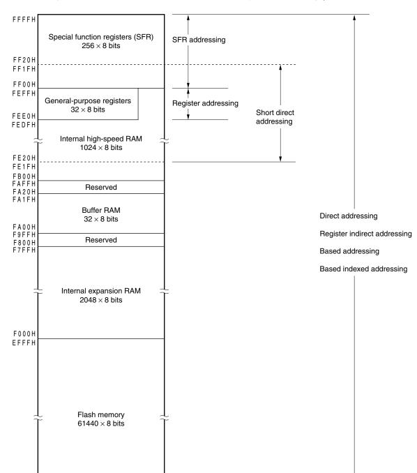
Figure 3-7. Correspondence Between Data Memory and Addressing (µPD78F0545)
