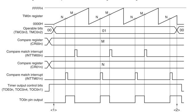
Figure 7-44. Example of Software Processing in Free-Running Timer Mode
