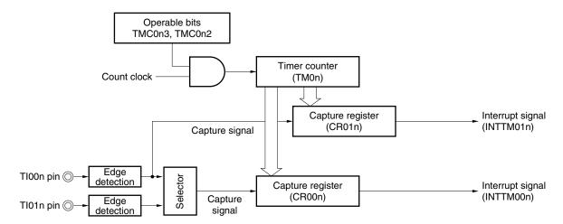
**Remarks 1.** If both CR00n and CR01n are used as capture registers in the free-running timer mode, the output level of the TO0n pin is not inverted.
