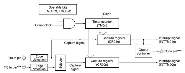
Note The timer output (TO0n) cannot be used when detecting the valid edge of the Tl01n pin is used.
