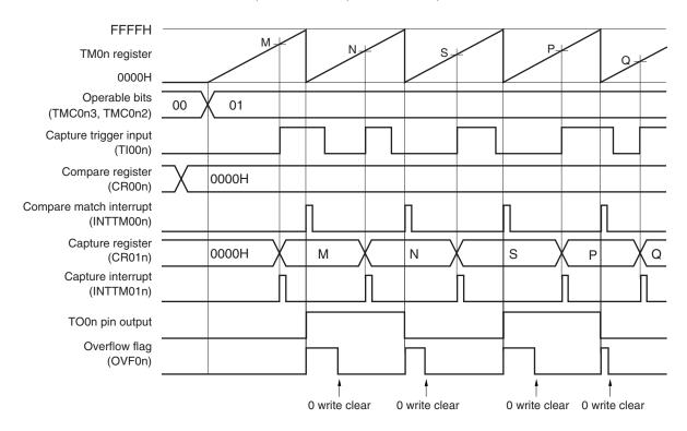
This is an application example where a compare register and a capture register are used at the same time in the free-running timer mode.
