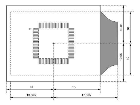
Figure B-1. For 80-Pin GC Package
