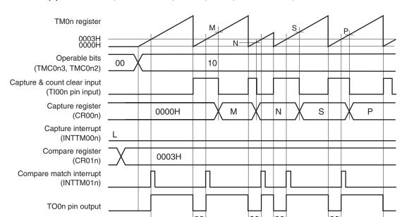
(b) TOC0n = 13H, PRM0n = 10H, CRC0n, = 03H, TMC0n = 0AH, CR01n = 0003H
