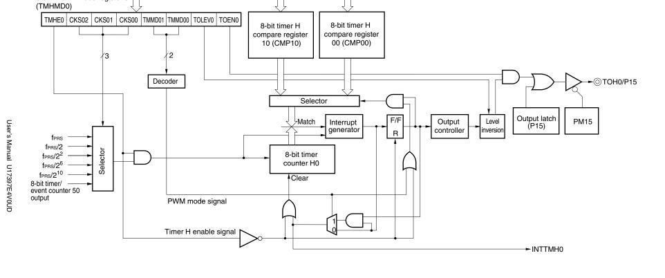
Figure 9-1. Block Diagram of 8-Bit Timer H0
