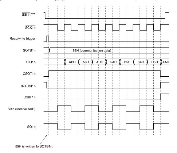
**Note** The SSE11 flag and SSI11 pin are available only for serial interface CSI11, and are used in the slave mode.
