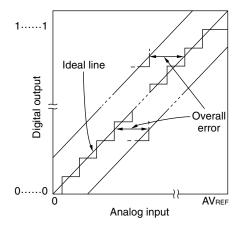
Figure 13-15. Quantization Error
