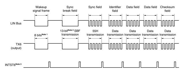
Figure 15-1. LIN Transmission Operation
