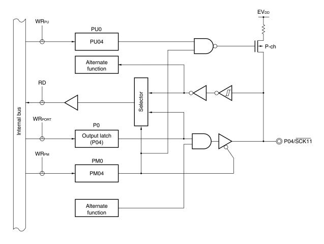
PU0: Pull-up resistor option register 0
