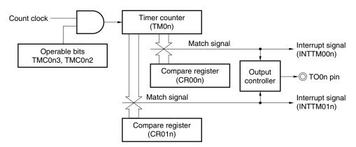
Figure 7-38. Timing Example of Free-Running Timer Mode (CR00n: Compare Register, CR01n: Compare Register)
