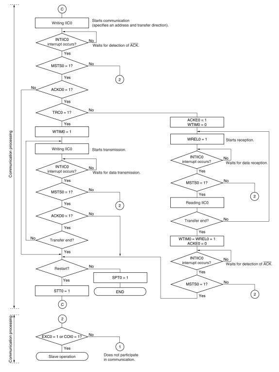
Figure 18-24. Master Operation in Multi-Master System (3/3)
