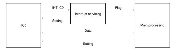
Therefore, data communication processing is performed by preparing the following three flags and passing them to the main processing instead of INTIICO.
