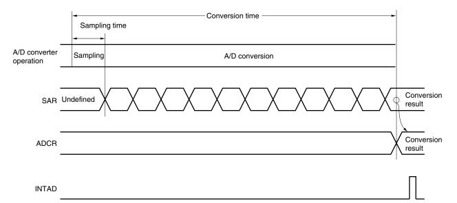
Figure 13-11. Basic Operation of A/D Converter
