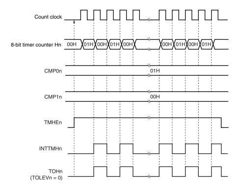
Figure 9-12. Operation Timing in PWM Output Mode (4/4)
