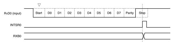
Figure 14-9. Reception Completion Interrupt Request Timing
