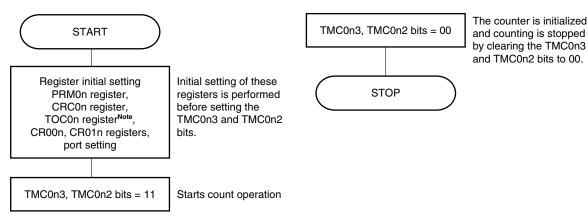
Note Care must be exercised when setting TOC0n. For details, see 7.3 (3) 16-bit timer output control register 0n (TOC0n).
