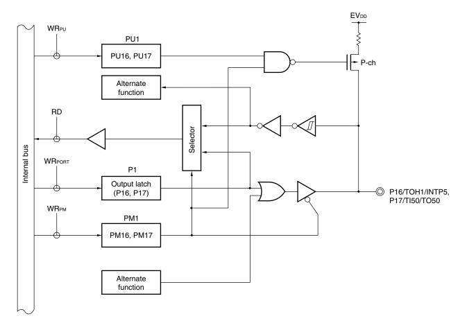
PU1: Pull-up resistor option register 1
