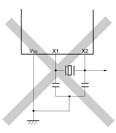
**Remark** When using the subsystem clock, replace X1 and X2 with XT1 and XT2, respectively. Also, insert resistors in series on the XT2 side.
