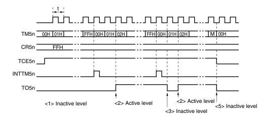
Remarks 1. <1> to <3> and <5> in Figure 8-14 (a) and (c) correspond to <1> to <3> and <5> in PWM output operation in 8.4.4 (1) PWM output basic operation.
