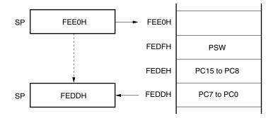
Figure 3-14. Data to Be Restored from Stack Memory
