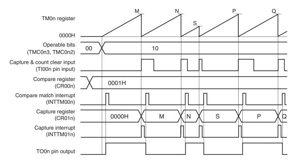
This is an application example where the output level of the TO0n pin is inverted when the count value has been captured & cleared.
