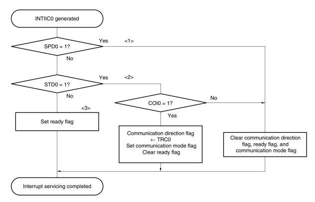
Figure 18-26. Slave Operation Flowchart (2)
