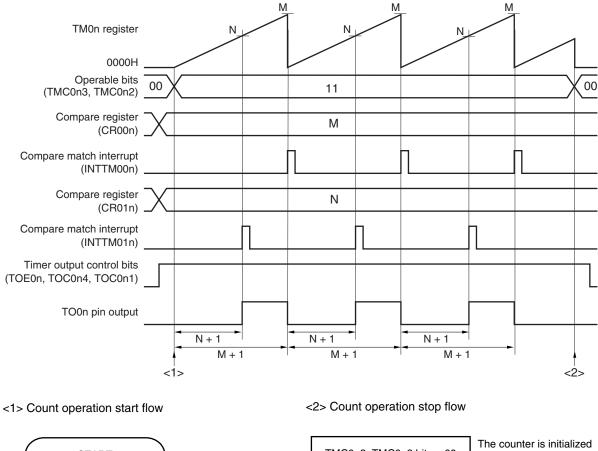
Figure 7-47. Example of Software Processing for PPG Output Operation
