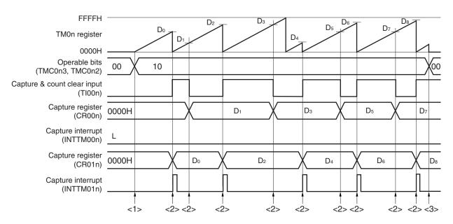
Figure 7-57. Example of Software Processing for Pulse Width Measurement (2/2)
