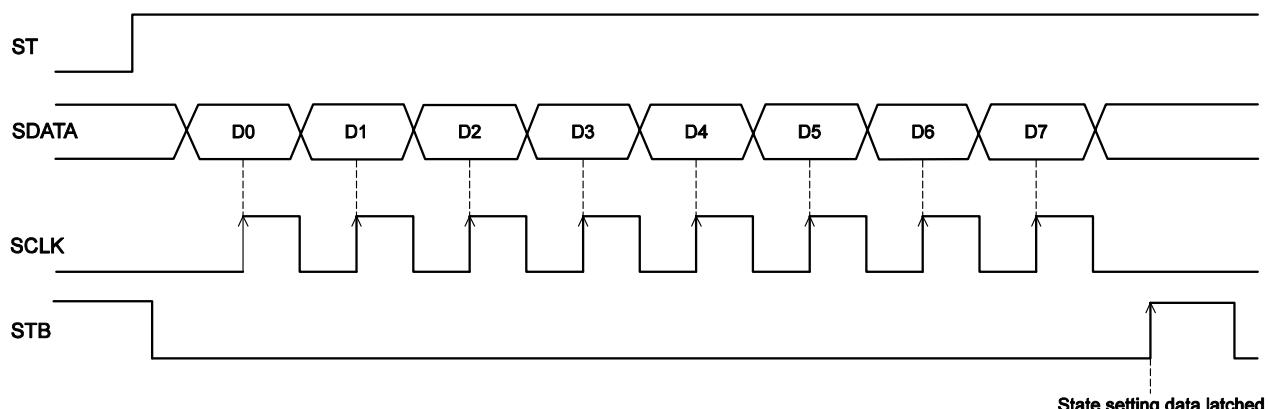
First set STB low and then input the SDATA and SCLK signals. The SCLK signal is not accepted when STB is high. SDATA inputs the data in the order D0, D1, ... D6, D7.
