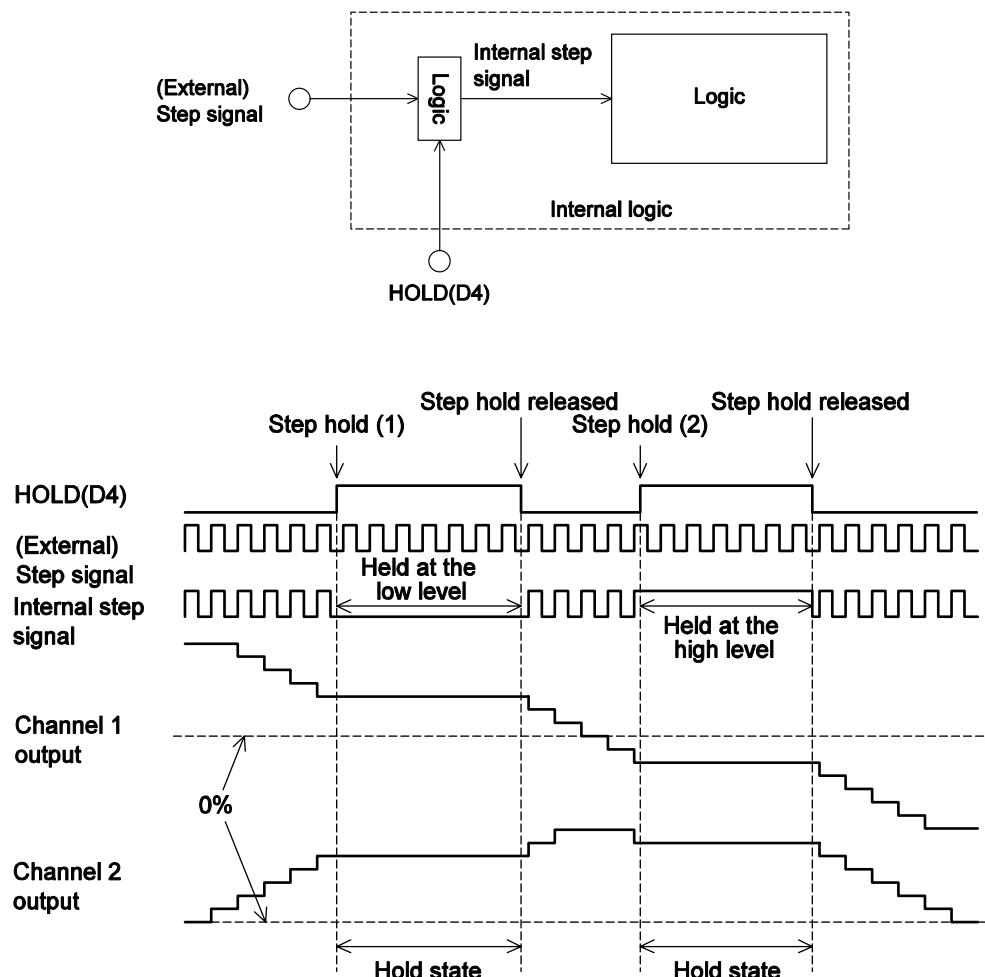
When the hold bit in the serial data, D4 (100, \*, D4, \*\*\*), is set to 1, the external step state at that time is held without change as the internal step state.
