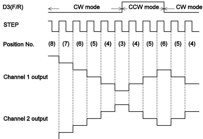
The IC internal D/A converter advances by 1 bits on the rising edge of the input step pulse.
