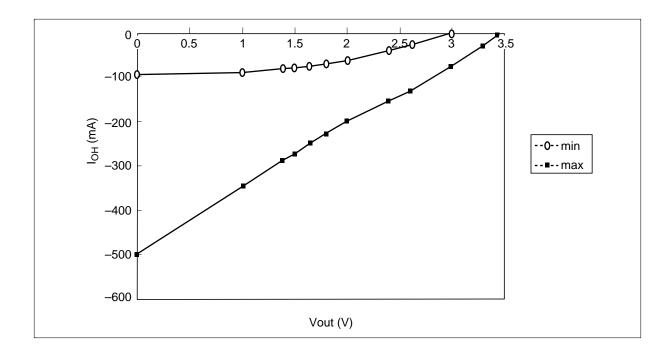
**DC Characteristics** (Ta = 0 to +70°C,  $V_{CC}$ ,  $V_{CC}Q = 3.3 \text{ V} \pm 0.3 \text{ V}$ ,  $V_{SS}$ ,  $V_{SS}Q = 0 \text{ V}$ ) (HM5225165B)
