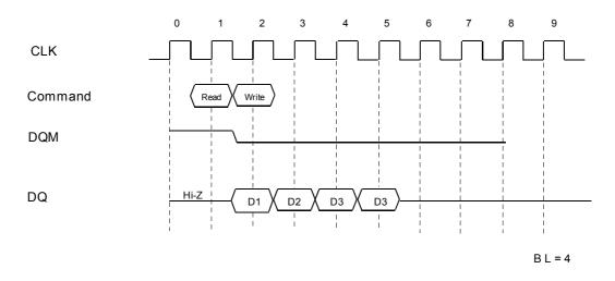
Read can be interrupted by Write. DQM must be high at least 3 clicks prior to the write command.
