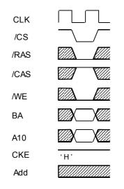
This command begins precharge operation of the bank selected by. When A10 is high,all banks are precharged, regardless of. When BA is low,only the bank selected by BA is precharged.
