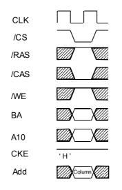
Raed data is available after /CAS latency requirements have been met. This command sets the burst start address given by the column.
