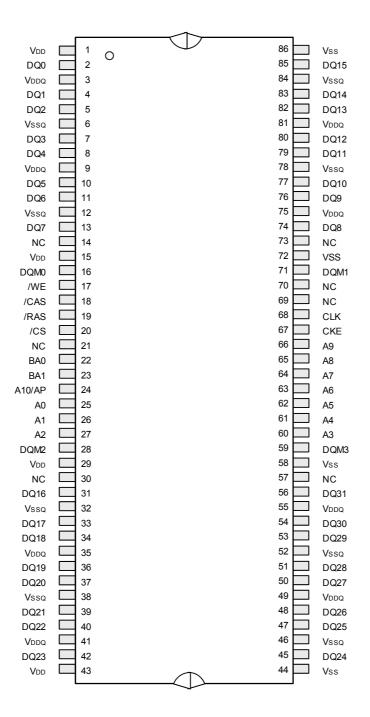
86pin TSOP-II (400mil x 875 mil) (0.5mm Pin pitch)
