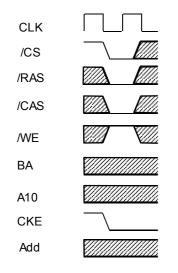
After the command execution, self refresh operation continues while CKE remains low. When CKE goes high, the memory exits the self refresh mode. During self refresh mode, refresh interval and refresh operation are performed internally, so there before is no need for external control. Before executing self refresh, both banks must be precharged.
