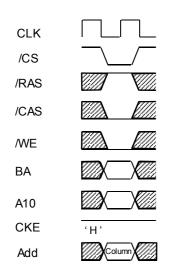
If the mode register is in the burst write mode, this command sets the burst start address given by the column address to begin the burst write operation. The first write data in burst mode can input with this command with subsequent data on following clicks.
