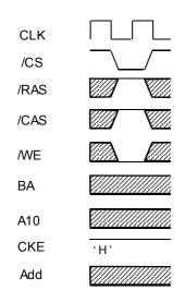
This command can stop the current burst operation.
