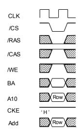
The EM482M3244VTA have 4 banks, each with 2,048 rows. This command activates the bank selected by BA and a row address selected by A0 through A10.This command corresponds to a conventional DRAM's /RAS falling.
