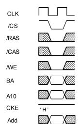
The EM482M3244VTA have a mode register that defines how the device operates. In this command, A0 through BA are the data input pins. After power on, the mode register set command must be executed to initialize the device. The mode register can be set only when all banks are in idle state. The EO482M3244VTA, cannot accept any other commands,only during 2CLK can following this command.
