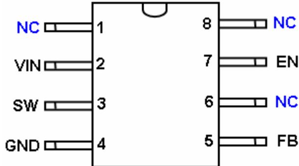
Figure 2 Pin Configuration of TD1583 (Top View)
