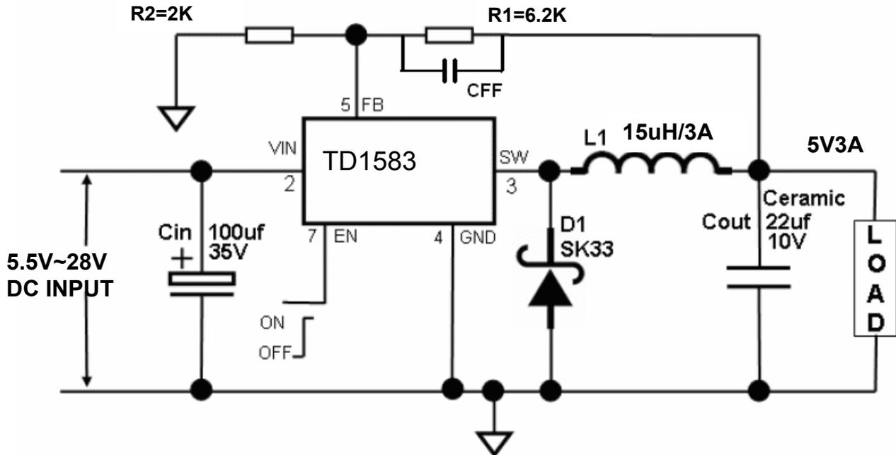
Fig10. TD1583 Typical Application Circuit (with ceramic output capacitor) @ 5V/3A
