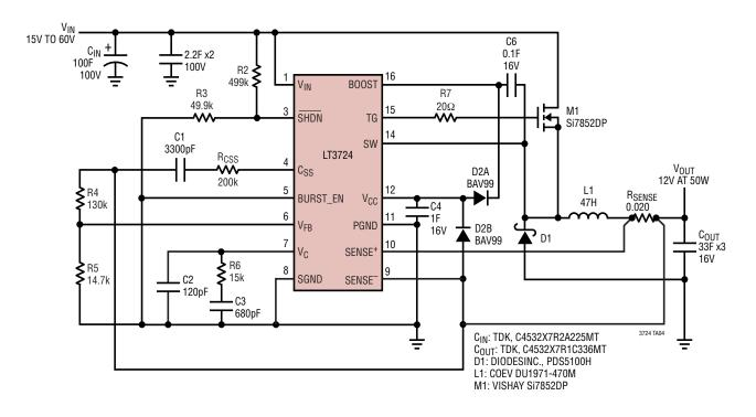
12V Step-Down with  $V_{CC}$  Back Driven from  $V_{OUT}$  and Ceramic Capacitor in Output Filter
