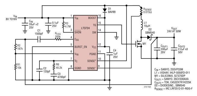
12V to 24V/50W Boost (Step-Up) Converter
