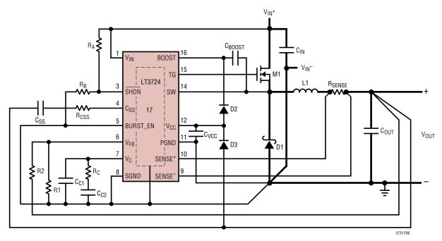
Figure 9. LT3724 Layout Diagram (See PCB Layout Checklist).
