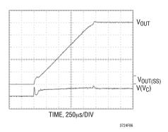
Figure 6. Desirable Soft-Start Characteristic
