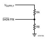
Figure 3. Undervoltage Lockout Circuit
