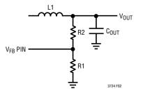
Figure 2. Output Voltage Feedback Divider
