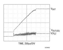
Figure 5. Soft-Start Characteristic Showing Excessive Ripple Component
