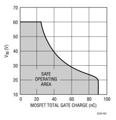
Figure 1.  $V_{CC}$  Regulator Continuous Operating Conditions
