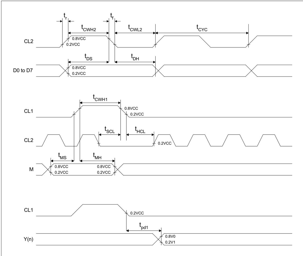
**Figure 8-2. AC Characteristics**
