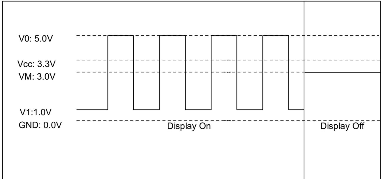
Figure 7-4. LCD Segment Drive Output Waveform & Voltage Level
