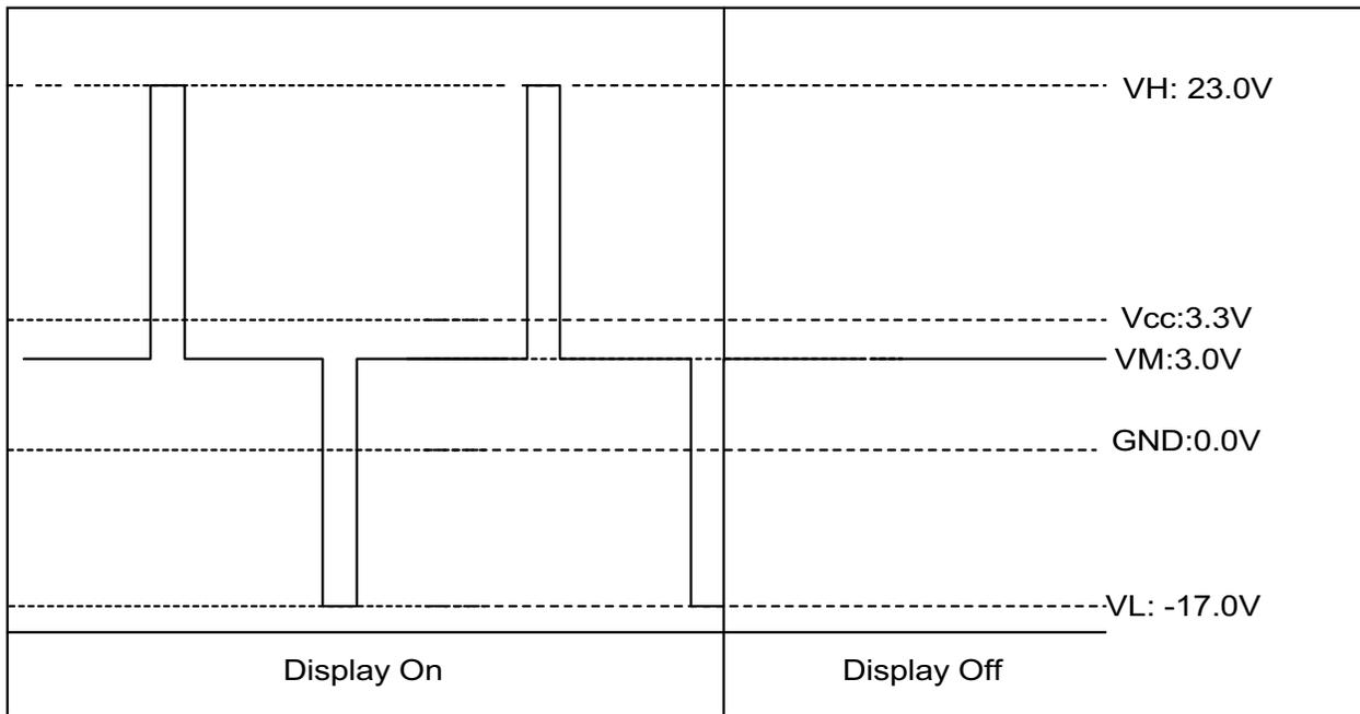
**Figure 7-3. LCD Common Drive Output Waveform & Voltage Level**
