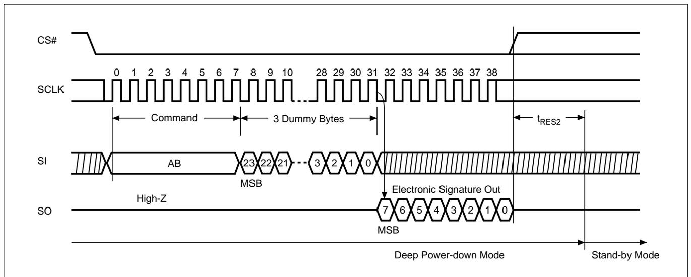
**Figure 24. Release from Deep Power-down (RDP) Sequence (Command AB)**
