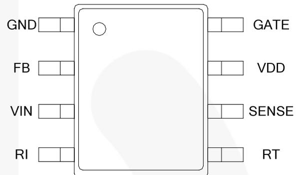
Figure 1. Pin Configuration
