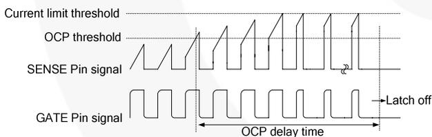
**Figure 14. Timing Chart for Two-level Over-Current Protection (OCP)**
