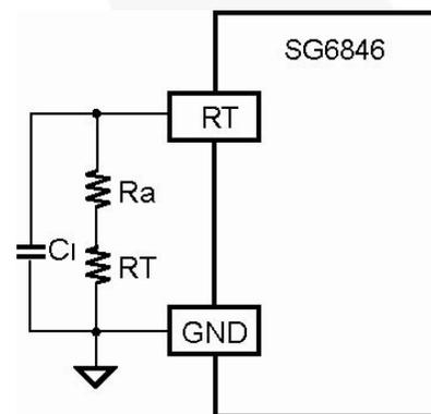
**Figure 15. T C1 (<1nF) Connect to RT Pin**
