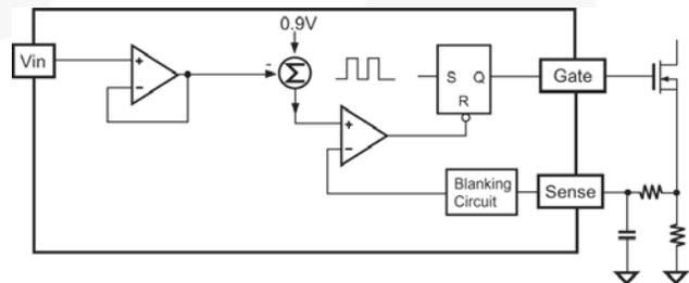
Figure 12. Universal Line Voltage Compensation for Constant Output Power Limit
