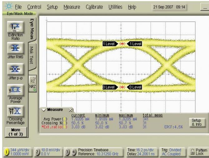
Figure 6: Eye diagram of the optical signal using the N4917A-E01 without any jitter added, measurement of ER and crossing point (PRBS  $2^{11}-1$  pattern)
