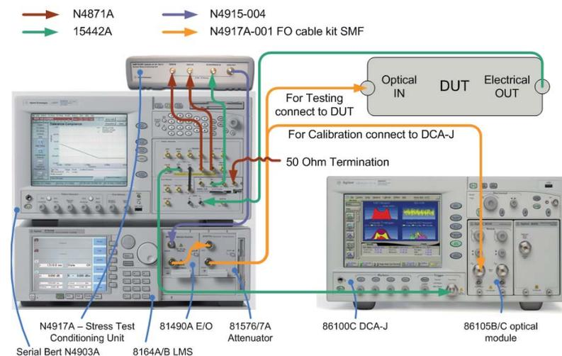
Figure 14: Setup for calibration including the recommended accessories
