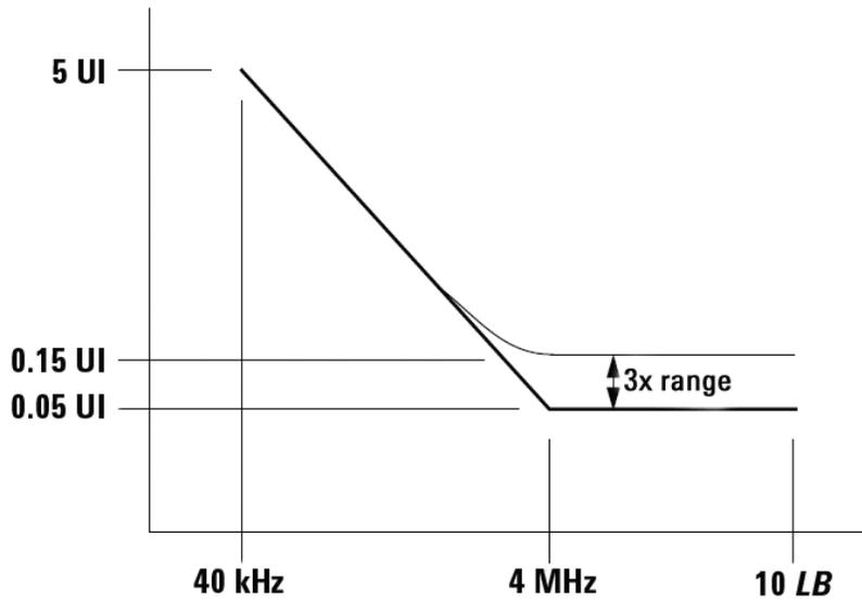
Figure 5: Jitter tolerance curve for 10 GBASE - LR/ - ER
