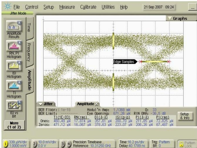
Figure 11: Amplitude measurement of the optical signal using the N4917A-E01 with 50 mUI periodic jitter and sinusoidal jitter added for a VECP of 2.2 (PRBS 2<sup>11</sup>-1 pattern)
