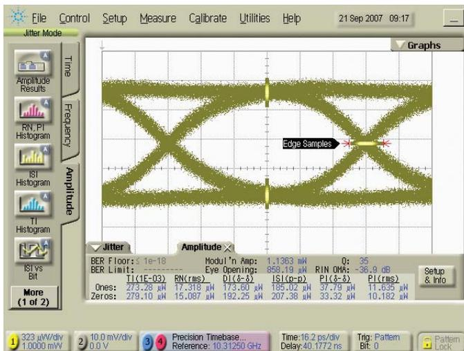
Figure 9: Amplitude measurement of the optical signal using the N4917A-E01 without any jitter added (PRBS 2<sup>11</sup>-1 pattern)
