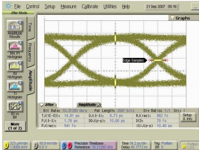
Figure 8: Jitter measurement of the optical signal using the N4917A-E01 without any jitter added (PRBS  $2^{11}-1$  pattern)
