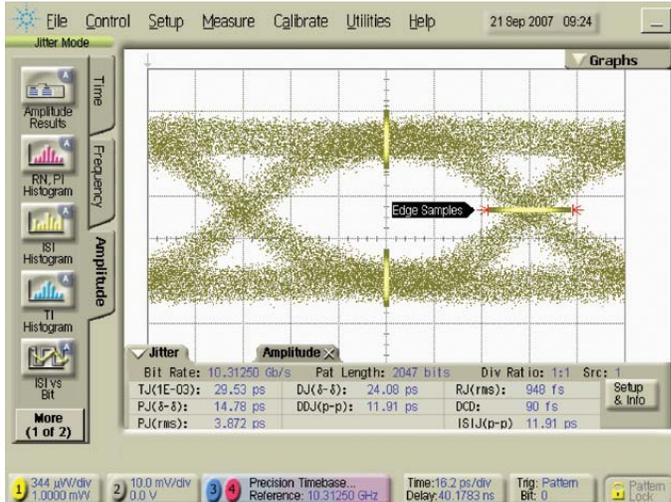
Figure 10: Jitter measurement of the optical signal using the N4917A-E01 with 50 mUI periodic jitter and sinusoidal jitter added for a VECP of 2.2 (PRBS 2<sup>11</sup>-1 pattern)
