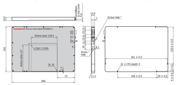
Top cover material including window is carbon fiber (1.0 mm thickness). Weight: 1.2  $\mbox{kg}$
