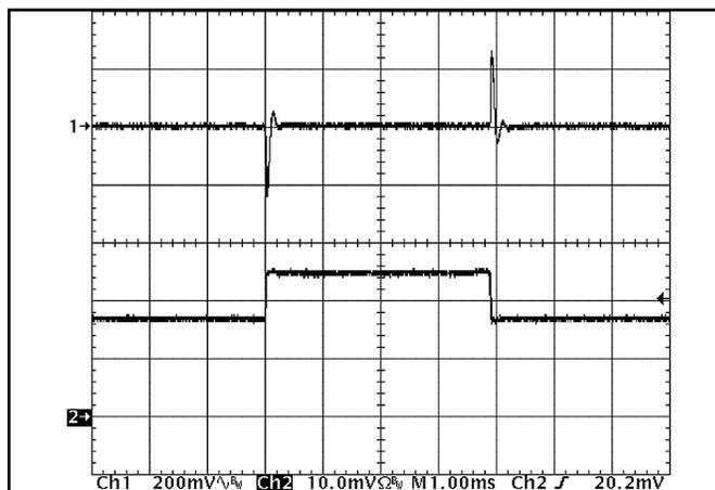
Figure 12: Output voltage response to step-change in load current (50%-75%-50% of  $I_{out(max)}$ ;  $dI/dt = 5A/\mu s$ ). Load cap: 480 $\mu F$ , 15 m $\Omega$  ESR tantalum cap and 1 $\mu F$  ceramic cap. Top trace:  $V_{out}$  (200mV/div), Bottom trace:  $I_{out}$  (10A/div).
