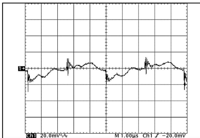
**Figure 16:** Output voltage ripple at nominal input voltage and rated load current ( $20\ \text{mV}/\text{div}$ ). Load capacitance:  $1\ \mu\text{F}$  ceramic capacitor and  $15\ \mu\text{F}$  tantalum capacitor. Bandwidth:  $20\ \text{MHz}$ . (See Figure 13)
