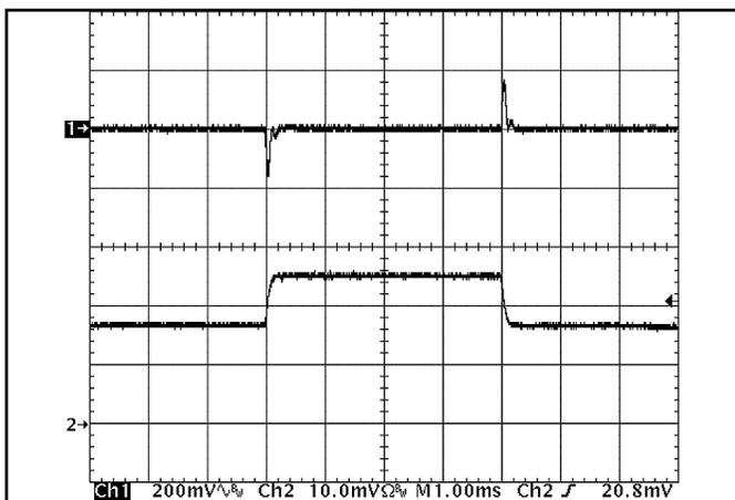
Figure 11: Output voltage response to step-change in load current (50%-75%-50% of  $I_{out(max)}$ ;  $dI/dt = 0.1A/\mu s$ ). Load cap: 15 $\mu F$ , 450 m $\Omega$  ESR tantalum cap and 1 $\mu F$  ceramic cap. Top trace:  $V_{out}$  (200mV/div), Bottom trace:  $I_{out}$  (10A/div).
