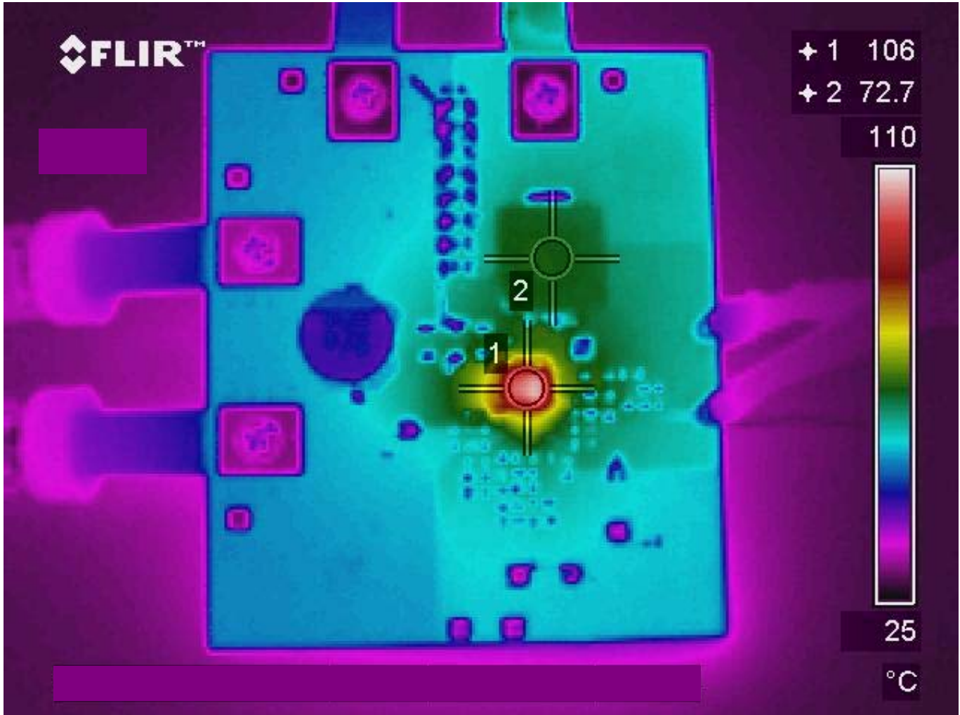
Fig. 17: Thermal Image at 14A load Test points 1 and 2 are IR3840A and inductor, respectively.
