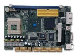
The HS-7238 is an Intel® 845GV GMCH/ICH4 chipset-based board designed. The HS-7238 series is ideal all-in-one PCI-ISA Bus single board computer. Additional features include an enhanced I/O with DVI-I/CRT, dual LAN, wireless LAN, audio and USB2.0 interfaces.
