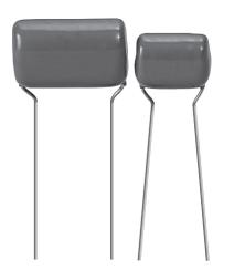
Contact Arc Suppression reduces field maintenance, premature equipment failure and RFI. A capacitor connected across the contacts helps in the solution of these problems but can cause contact welding and reduced equipment reliability. By adding a resistor in series with the capacitor, these additional problems are eliminated.
