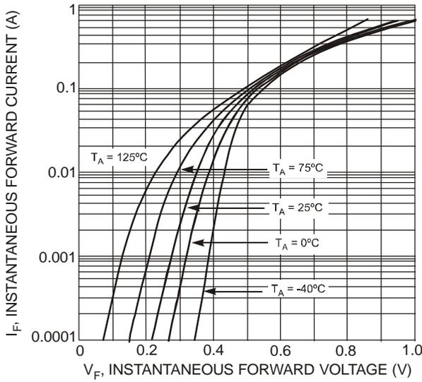
Fig. 1 Forward Characteristics
