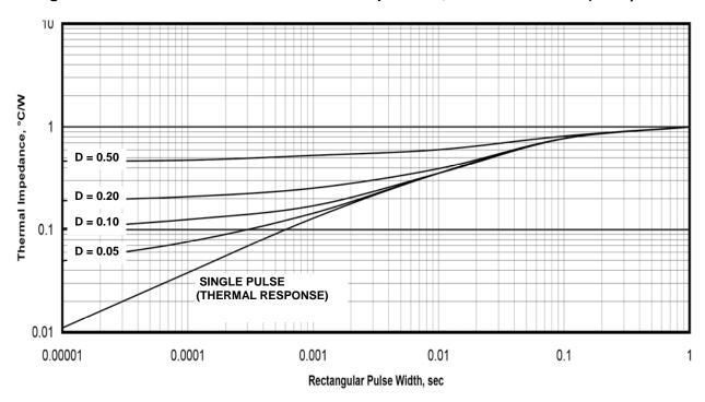
Figure 5. Normalized Transient Thermal Impedance, Junction-to-Case (Diode)
