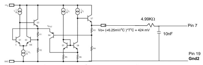
Fig. 6 Temperature Sensor Internal Block Diagram
