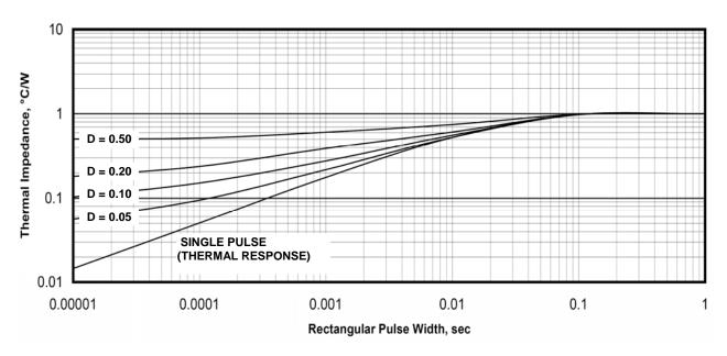
Figure 4. Normalized Transient Thermal Impedance, Junction-to-Case (IGBT)
