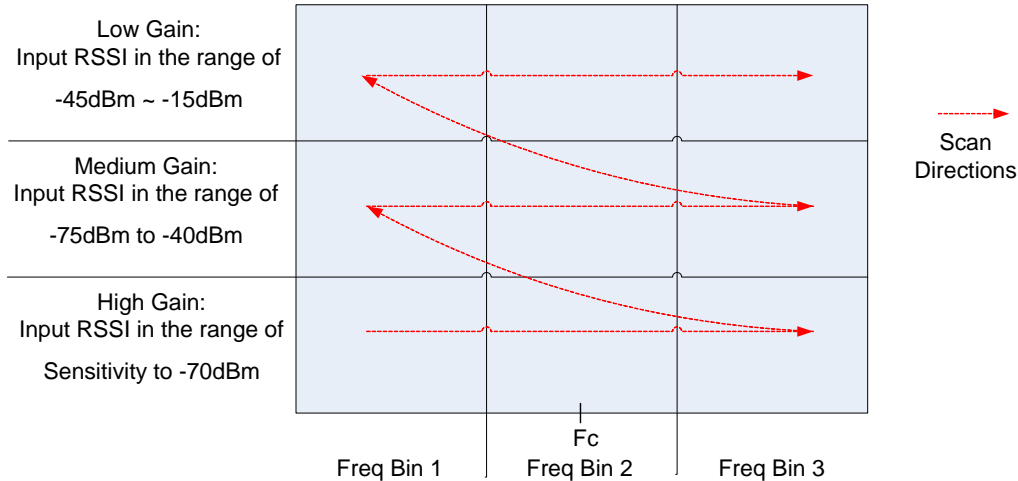
Figure 6. Frequency Scan Algorithm Depicting 3 Frequency Bins of 140 kHz and 3 Gain Settings
