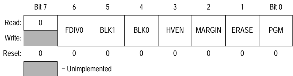
Figure 4-1. FLASH 2TS Control Register (FLCR)
