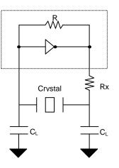
$\begin{aligned} C_L &= 2^*(C_P - C_S), \\ Where & C_P = Load \ capacitance \ of \ crystal \\ & C_S = Stray \ capacitance \ due \ to \ C_{IN,} \ PCB, \ Trace \ etc. \end{aligned}$
